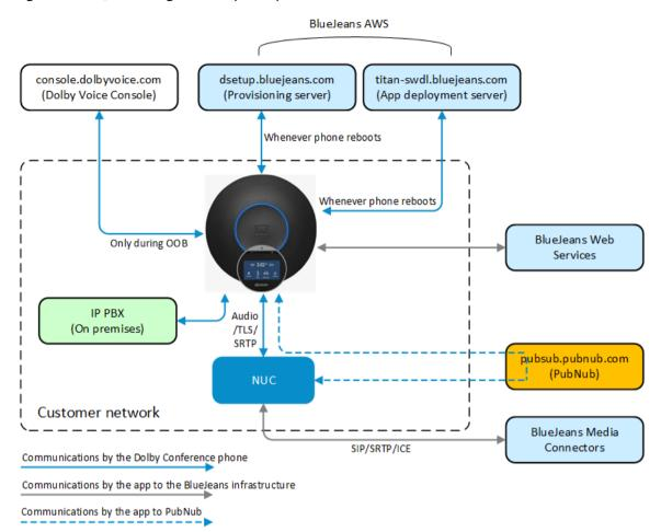
Figure 1: BlueJeans Plug-and-Play Setup Architecture
